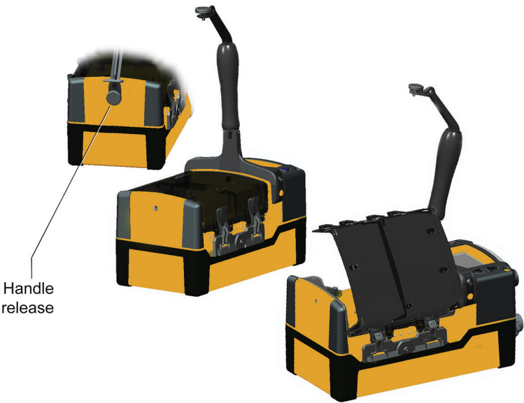
Figure 8: Opening the Chemcassette cartridge door
