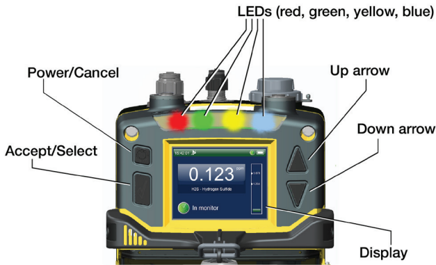
Figure 2: SPM Flex buttons and color LCD display
