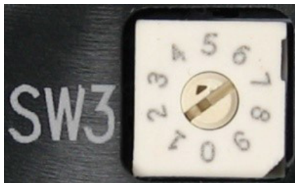
Figure 26. Ten-position rotary switch SW3.
