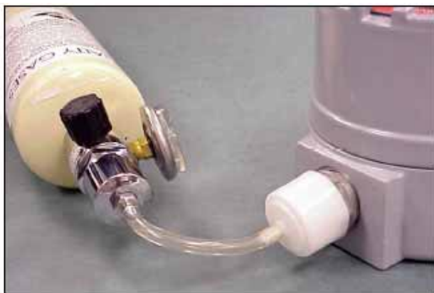
RaeGuard connected to gas bottle with Calibration adapter
